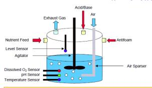
Bioreactors are large vessels that serve as an environment for biochemical reactions to occur. Typical uses include the growth of microorganisms and the breakdown of products.
